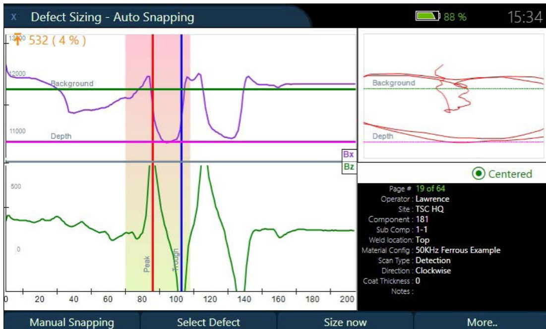
Figure 13 Defect Sizing – Auto Snapping
